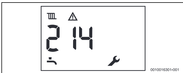
Fig. 104 Example: non-blocking fault
